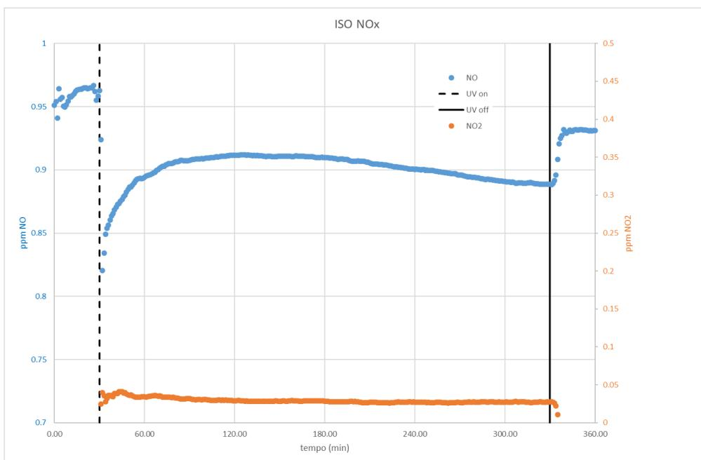
Considering the results obtained, it is possible to calculate, by numerical integration, that **the Calacatta SL Active 2.0 - 300x150 cm sample degrades 2.4 mg of NO per square meter of material** for each hour of work.
